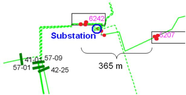
Fig.4. Result of fault location during operation (case I)
