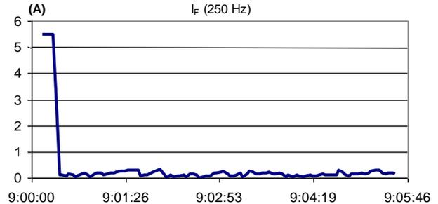
Fig.14. Field test results for 5th harmonic fault current compensation
