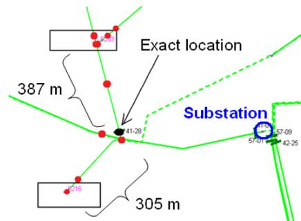
Fig.5. Result of fault location during operation (case II)
