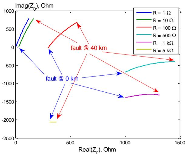
Fig.2. Calculated zero sequence impedances for various fault locations and fault resistances at a 40 km line
