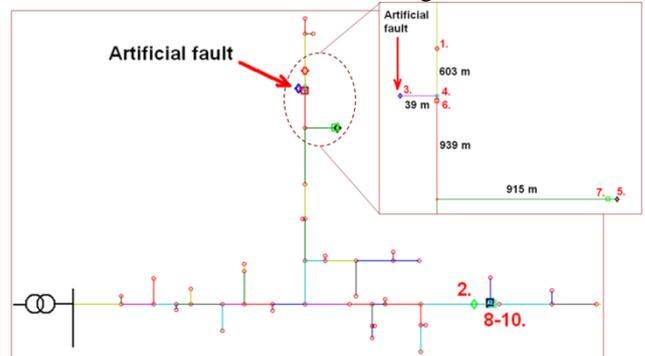
Fig.3. Result of fault location in a MV network field test
